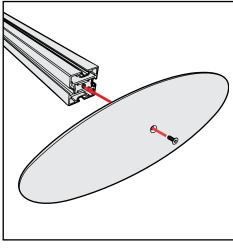
Base Plate & Extrusion Connection
