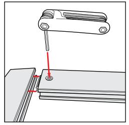
Extrusion & Lock Connection
